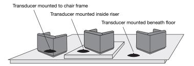
NOTE: Transducers are designed to be mounted in a horizontal orientation. Mounting the Transducer vertically may shorten the Transducer's life.
