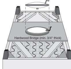
Transducer mounts on hardwood bridge attached to chair frame, or to a centrally-located frame member, if present.
