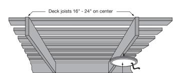
TST mounts directly to bottom of joist using Hanger Bolt
