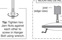
For use with metal or some other high-tensile mounting surfaces no thicker than 1/4". Requires access to the top of the mounting surface both to install the bolt and to tighten it.
