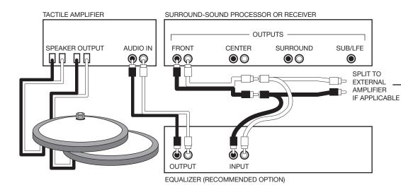
**NOTE:** If you are using a surround-sound receiver with built-in amplifiers, you <u>DO NOT</u> need to split the FRONT output as shown in this diagram.
