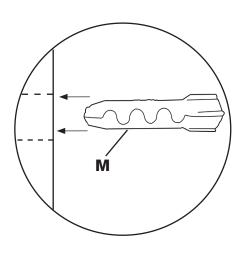
C Insert wall anchors (M) into hole.
