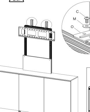
Loosely mount Bracket (O) using Screw (C), Washer (M) and Drop-In Nut (B).
