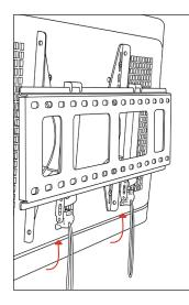
Center tv brackets on wall bracket and push black click fasteners Up into lock position.
