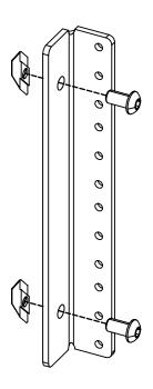
**2** Place the Rack Rail into position with the Drop-in Nuts (vertically) sliding into the channel as shown. After bracket is in position tighten all screws with Hex Key.
