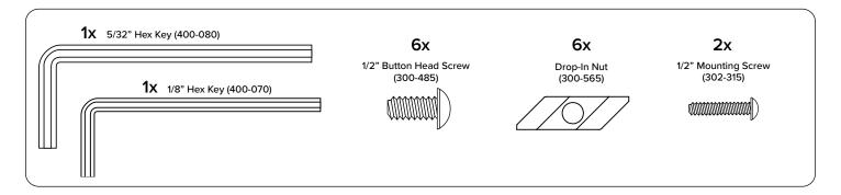
1 Place the 1/2" Button Head Screw (300-485) through the rack rail and loosely screw to Drop-In Nut (300-565).
