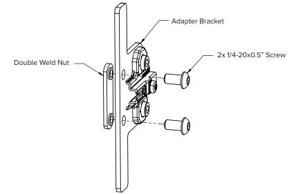
**B.** On each side of the bay the drop down door will be installed in, slide the double weld nut of the adapter plate assembly into the inner slot of the extrusions as shown. Once the adapter plate assembly is resting on the bottom, tighten the screws to secure the assemblies in place.
