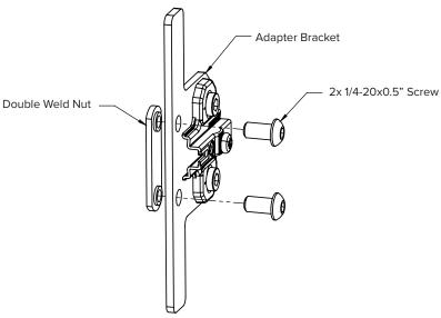
**B.** On each side of the bay the drop down door will be installed in, slide the double weld nut of the adapter plate assembly into the inner slot of the extrusions as shown. Once the adapter plate assembly is resting on the bottom, tighten the screws to secure the assemblies in place.
